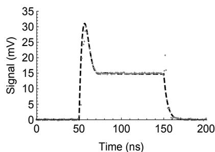
Transient measurement of 20 mM TEMPO in hexane at room temperature *during* a kW pulse. The data shows both experiment and fit assuming an effective  $T_1 = 20$  ns and  $T_2 = 4$  ns.
