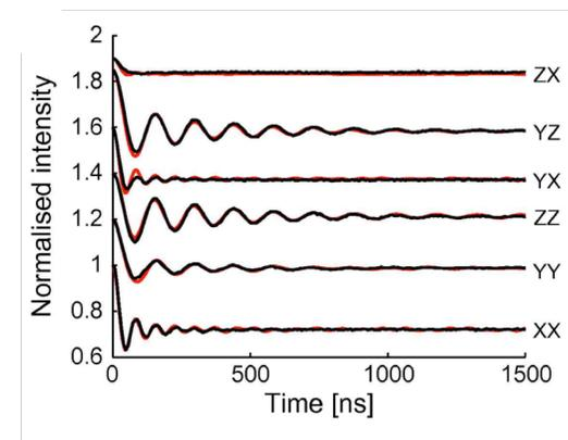
Orientational PELDOR measurements on a bis-nitroxide model system in o-terphenyl. This highly constrained data set, obtained over 500 MHz bandwidths allows both distance and orientational distributions to be derived.
