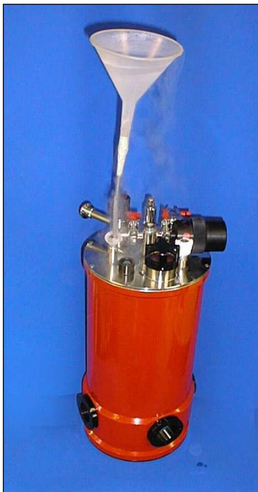
**Photo 3.1.** Using a funnel to fill a cryostat with liquid nitrogen
