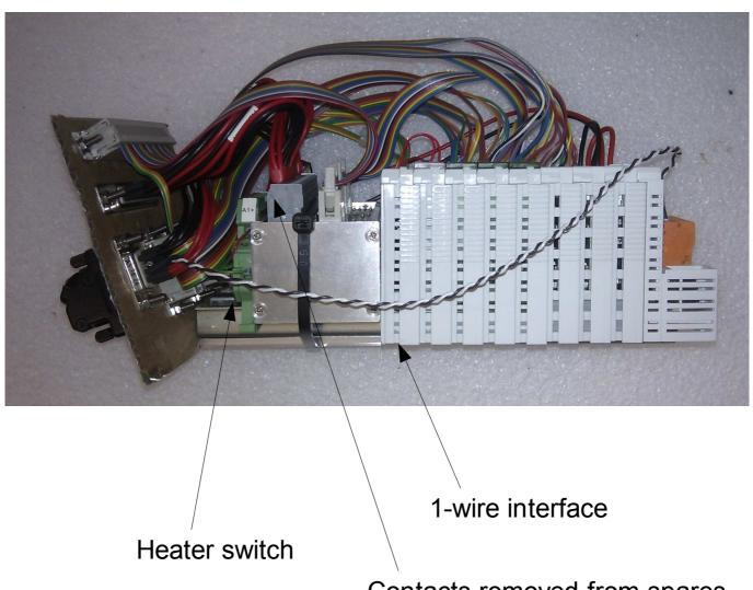
Contacts removed from spares of these connectors to make the 1-wire interface
