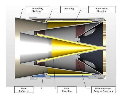
Figure 1: Cross-section view of the hot calibration load, from [RD4].
