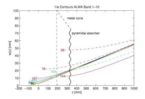
Figure 2: – ALMA beam sizes as a function of frequency
