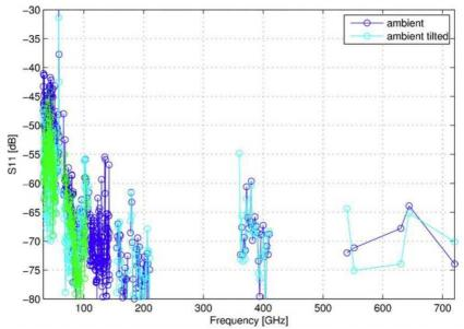
Figure 5: S11 performance of prototype ambient calibration load, from [RD3] / [RD4].
