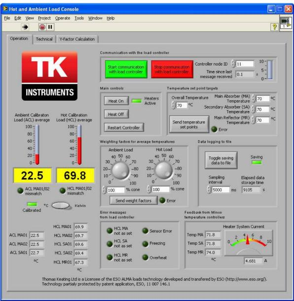
Figure 11: front panel of hot and ambient load console application. Square green 'LED' indicators have been used to show correct operation. Round pink 'LEDs' indicate errors or warnings, along with the "time since last message received" tank which will fill up if there is a communications problem.
