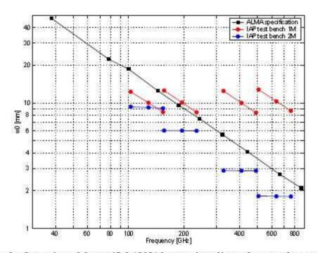
Figure 1: Comparison of the specified ALMA beam waist radius at the center frequencies of Band 1 to 10 (black squares) with the accessible beam waists of the IAP setup using one (red) or two (blue) focusing reflectors. Measurements below 100 GHz were made with the original ALMA feed horns and lens antennas. In the overlap region at 100 GHz measurements were made with the ALMA and the IAP optics, which resulted in consistent results.
