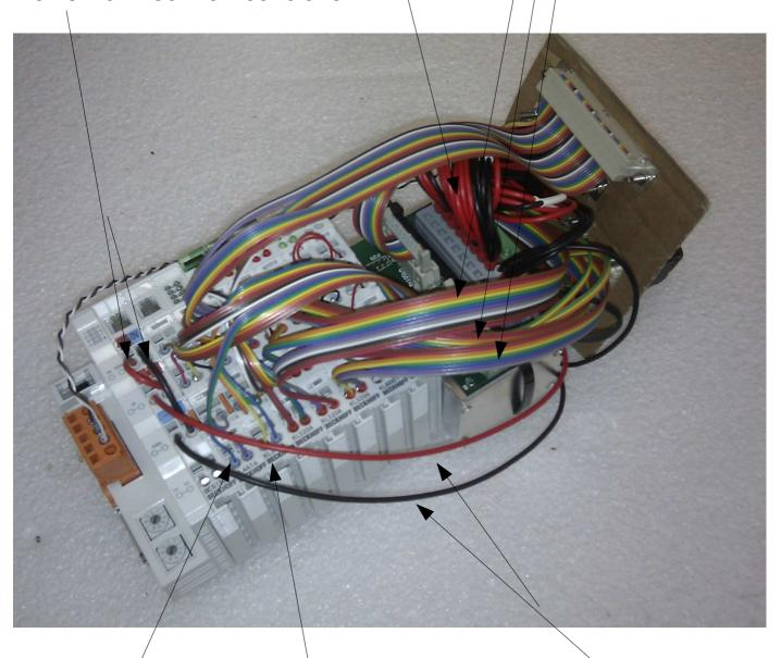
Current source with 4 outputs all to Minco box one of which switches power to all heaters
