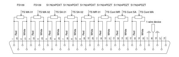
Figure 17: Hot load sensors connector.
