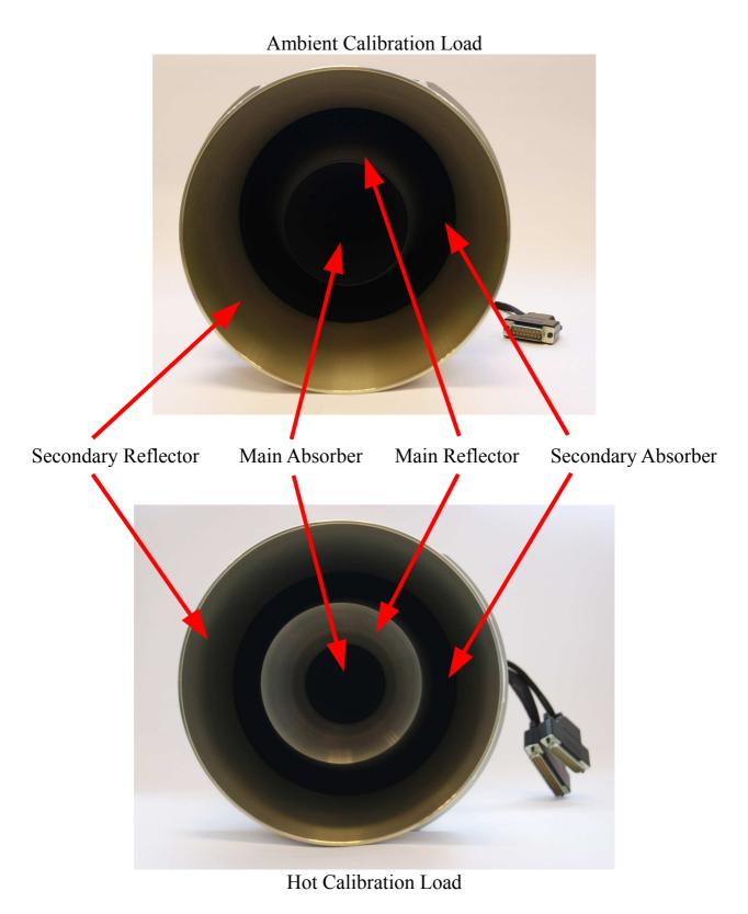
Figure 7: Photographs of the ambient and hot calibration loads with the absorbing and reflecting components labelled.
