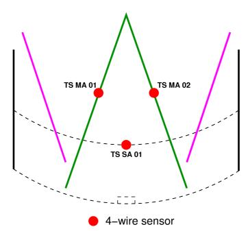
Figure 8: Sketch of the sensor locations in the ambient load.
