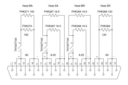
Figure 18: Hot load heaters connector.
