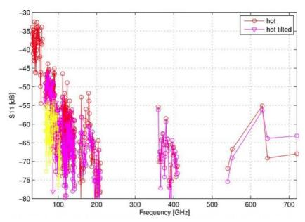
Figure 6: S11 performance of prototype hot calibration load, from [RD3].
