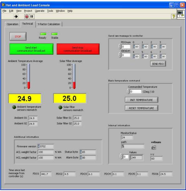
Figure 12: technical panel of hot and ambient load console application.
