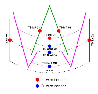
Figure 9: Sketch of the sensor locations in the hot load.
