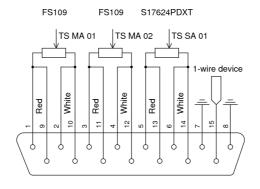
Figure 16: Ambient load sensors connector.
