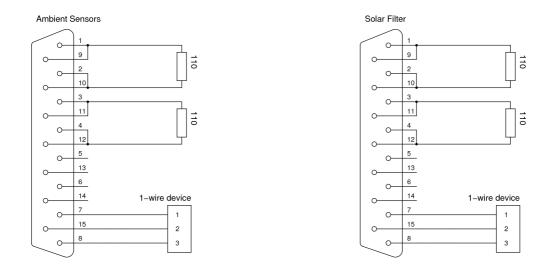
Figure 15: Schematic of dummy connectors. The  $110\Omega$  resistors could be replaced with PRT100 sensors to add additional readout channels.
