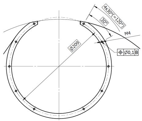
Figure 10: Drawing of the mechanical interface of the calibration wheel where a calibration load is mounted.
