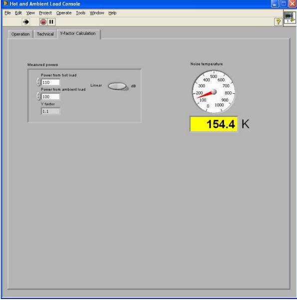
Figure 13: Y-factor calculation panel.
