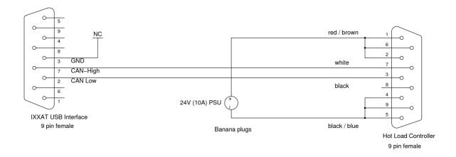
Figure 14: Schematic of power / CAN cable.
