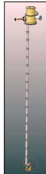
TK has manufactured two 94 GHz probes for ESR and DNP-NMR, using two refocussing mirrors to feed the beam to the sample holder from below, allowing a sample changer mechanism to extract the sample from above.
