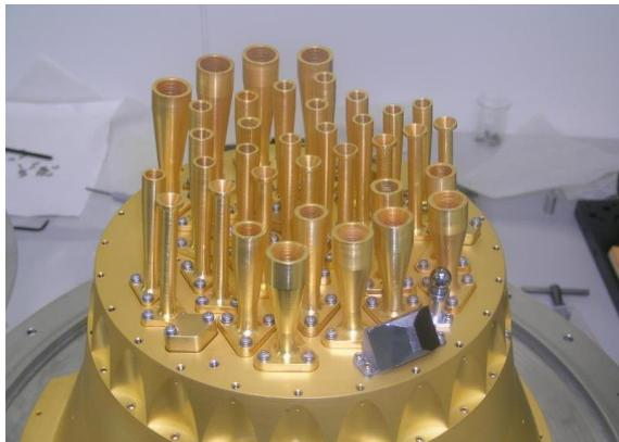
The feed-horn cluster for the Planck High Frequency Instrument, now parked near Lagrangian point L2
