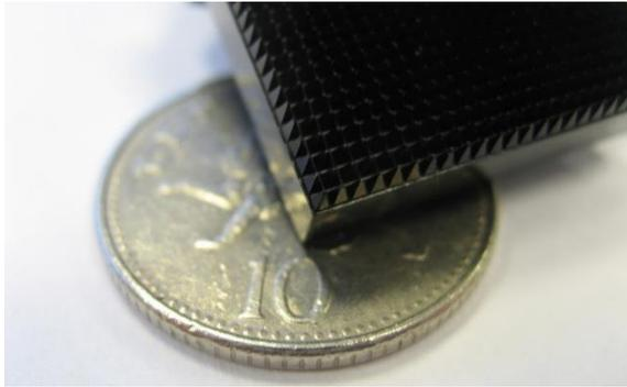
TK RAM tile with sharp pyramidal array: 25 mm square for higher frequencies
