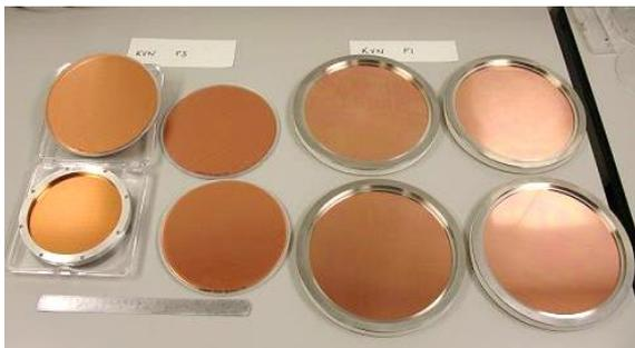
Free-space multi-mesh filters with a 30 cm rule for scale.
