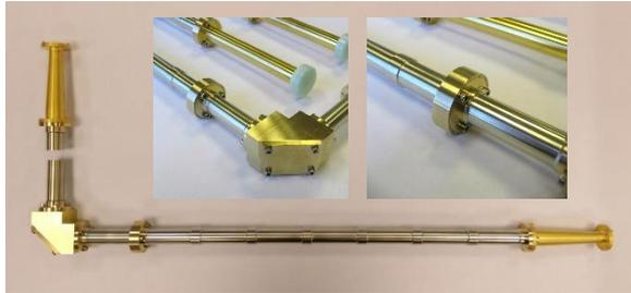
18 mm ID 263 GHz corrugated waveguides with precision mitre bends, rotatable flanges and tapers. Larger and smaller IDs and a larger range of frequencies are available.
