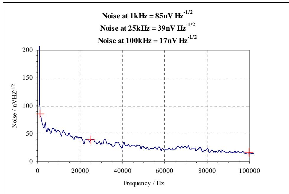
**Fig. 6.2.** System output noise spectrum
