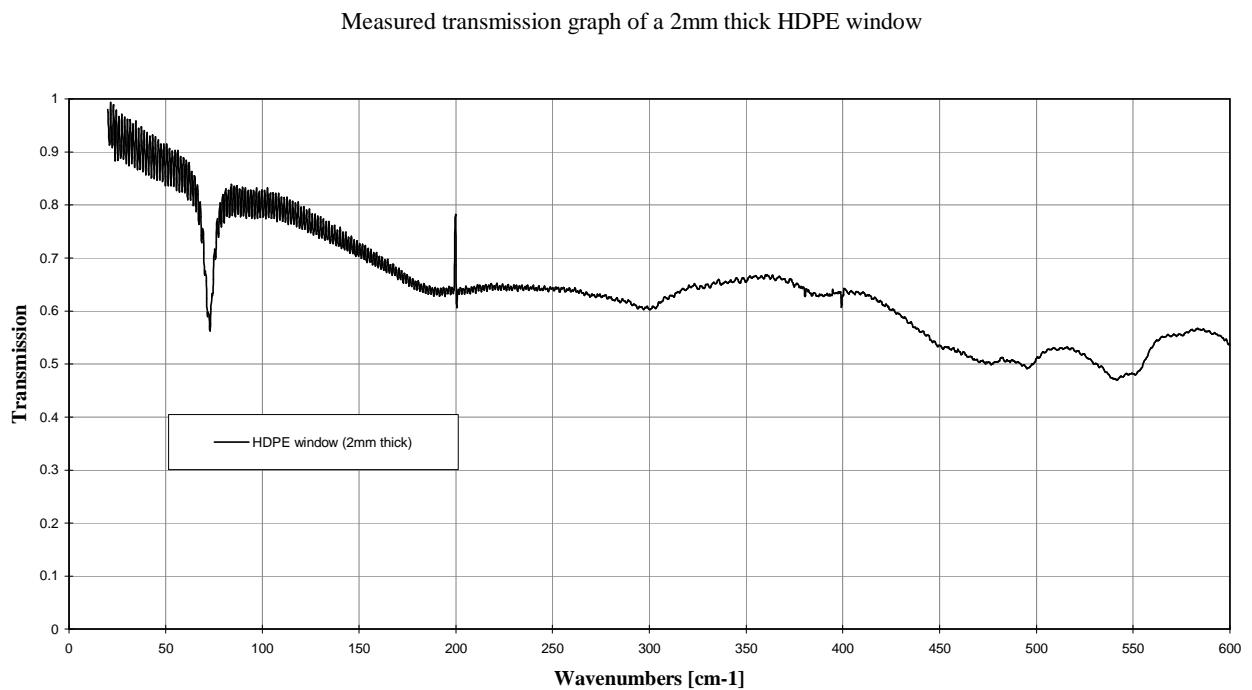
**Fig. C.2.** Measured transmission of a 2mm thick HDPE window from  $20\text{cm}^{-1}$  to  $600\text{cm}^{-1}$ .
