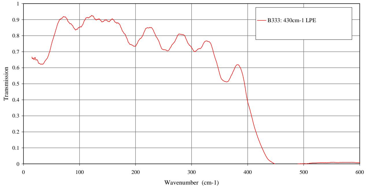
Fig C.1. Transmission spectrum for the type QMMF  $430\text{cm}^{-1}$  low pass filter
