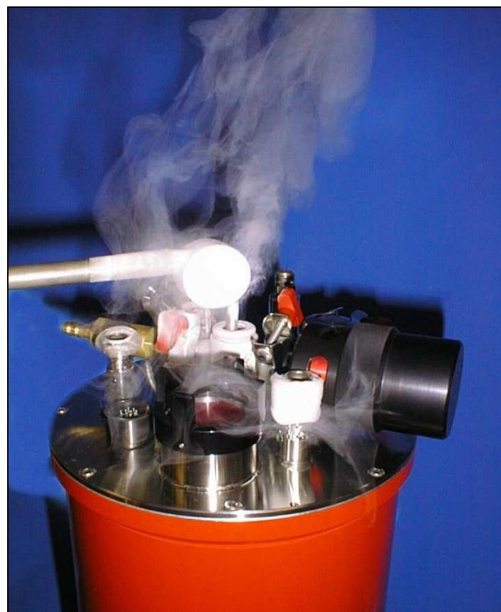
**Photo 4.2.** Helium gas exhaust during fill
