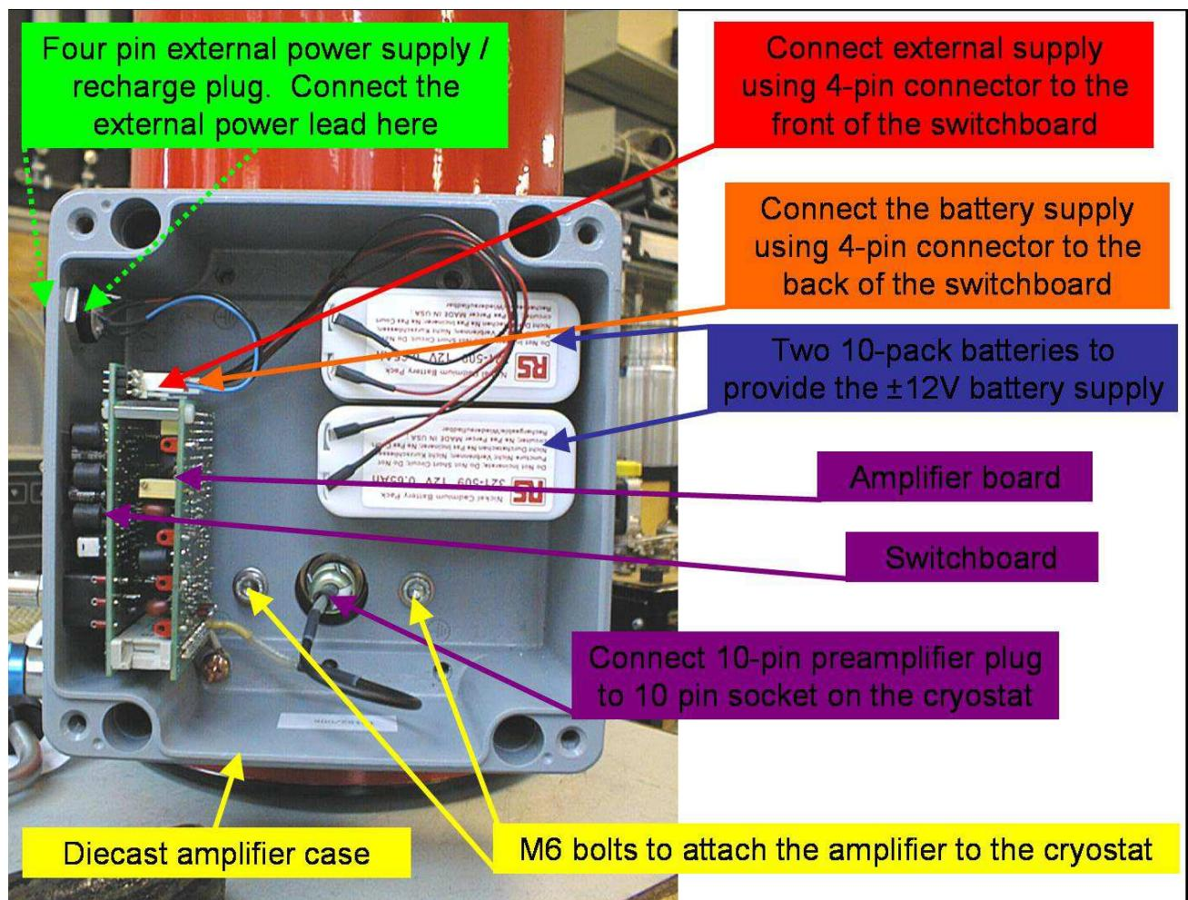
**Photo 5.1a.** Mounting the preamplifier to the cryostat
