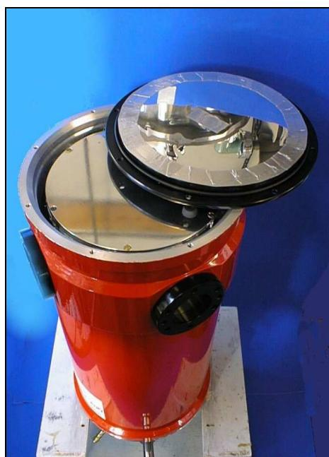
**Photo 1.4.** Liquid nitrogen base-plate in position
