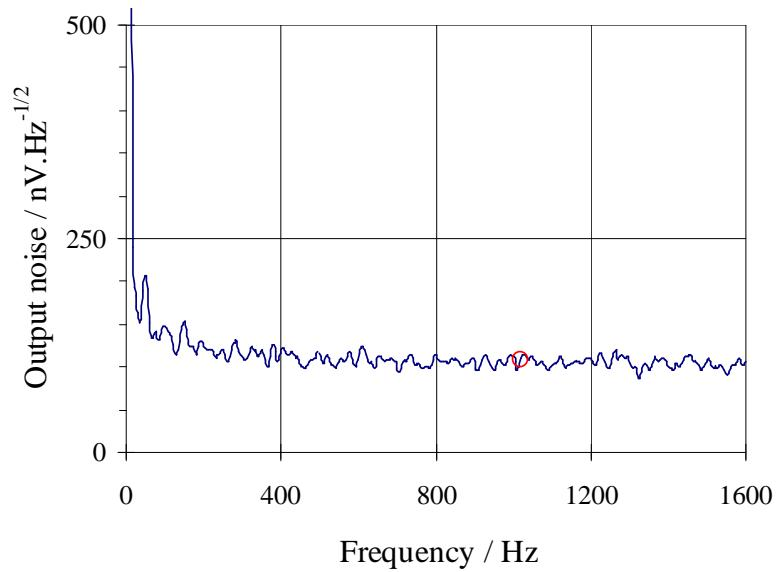
**Fig. 5.1a.** Typical preamplifier input shorted noise spectra at low frequencies
