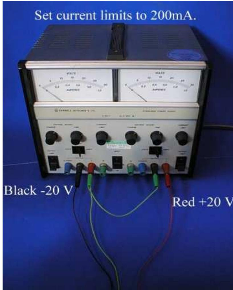
**Photo 5.2.** Power supply connections
