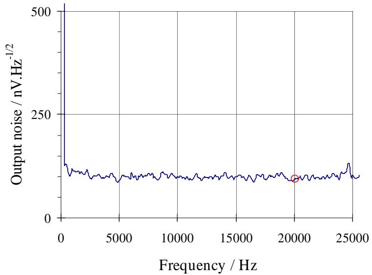
**Fig. 5.1b.** Typical preamplifier input shorted noise spectra at higher frequencies
