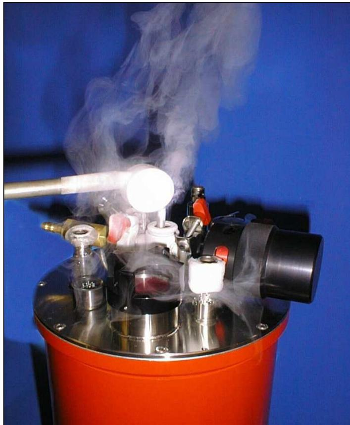
**Photo 4.2.** Helium gas exhaust during fill
