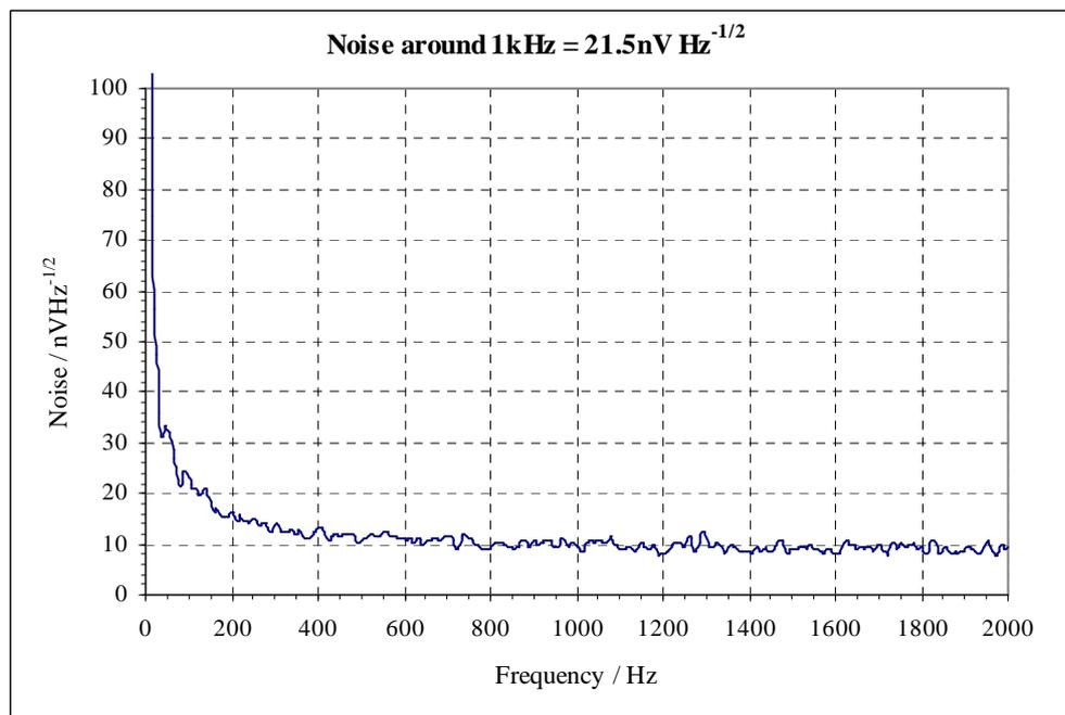
**Fig. 6.2.** System output noise spectrum. 0 to 2000Hz
