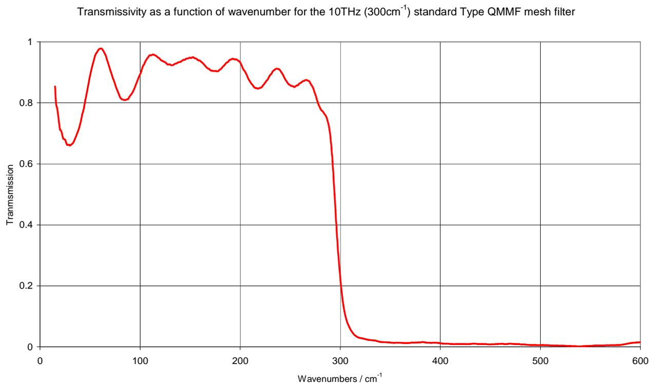
**Fig. C1.** Transmission spectrum for the type QMMF  $300\text{cm}^{-1}$  low pass filter
