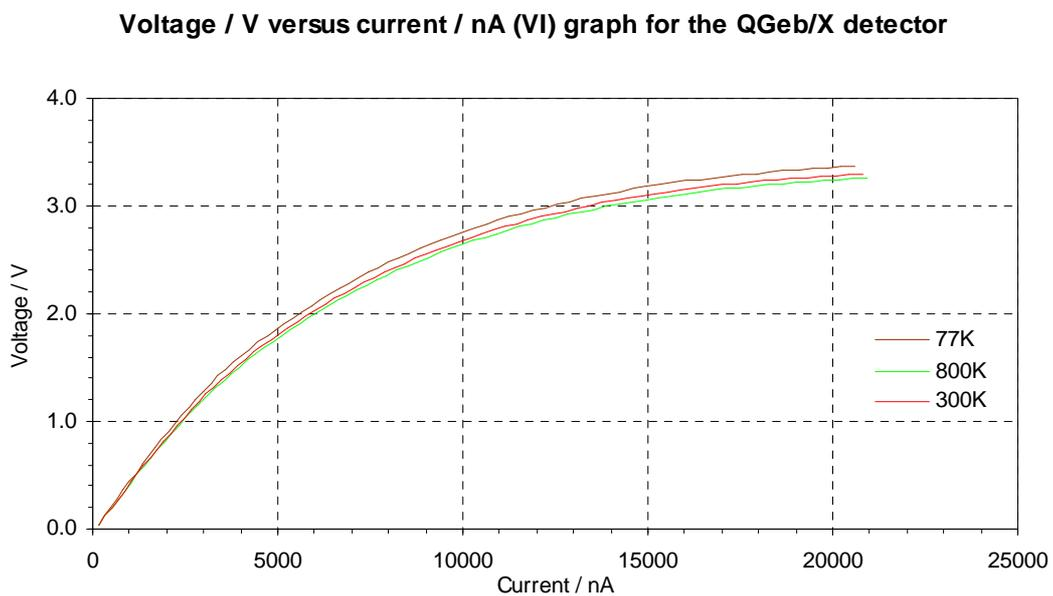
**Figure A1.** The detector VI characteristic measured through  $300\text{cm}^{-1}$  low-pass filtering with an 800K, 300K and 77K dc load.
