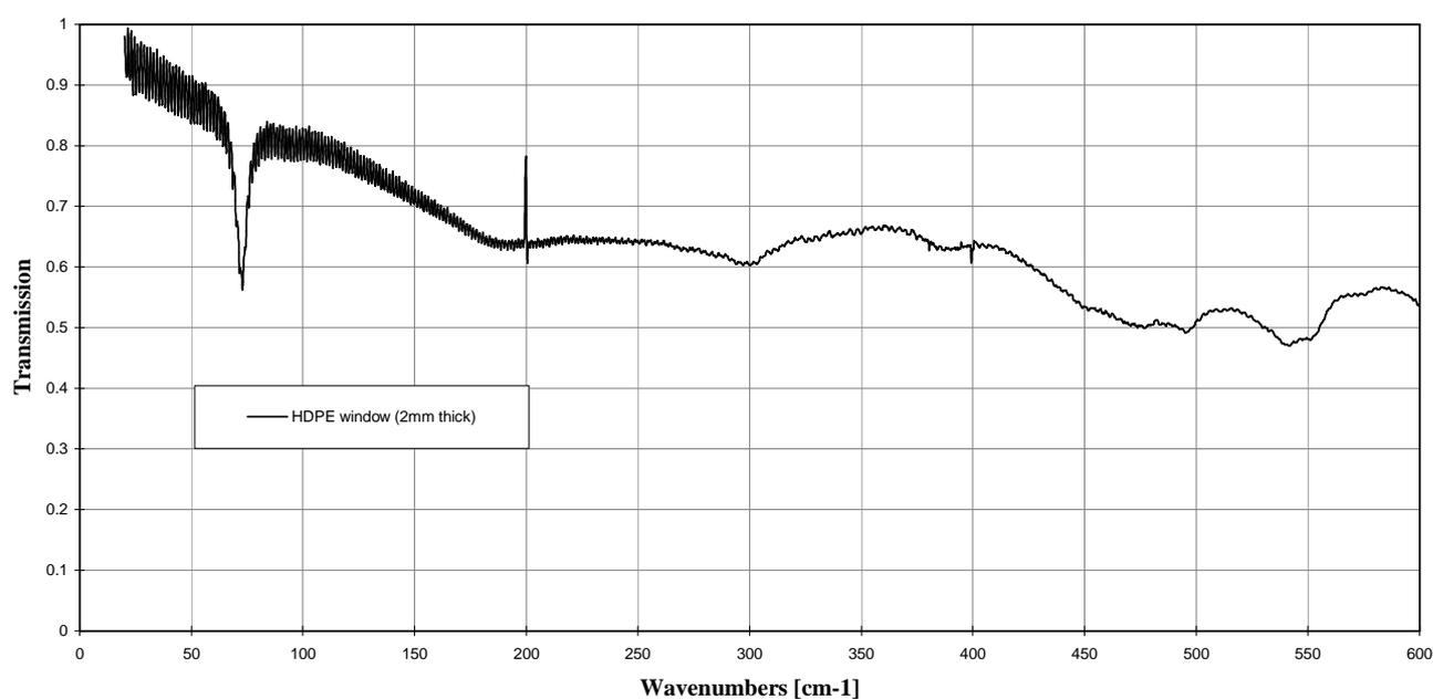
**Fig. C.2.** Measured transmission of a 2mm thick HDPE window from  $20\text{cm}^{-1}$  to  $600\text{cm}^{-1}$ . The polyethylene characteristic absorption increase is clearly seen around  $73\text{cm}^{-1}$
