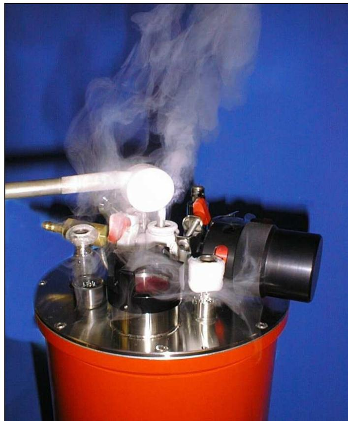
**Photo 4.2.** Helium gas exhaust during fill
