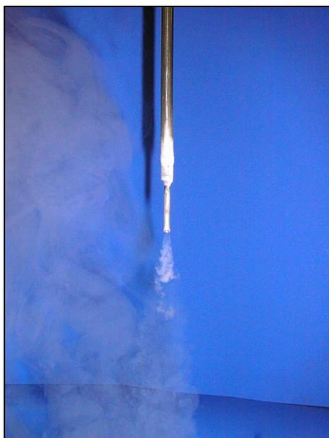
**Photo 4.5.** Liquid helium emerging from a cold tube
