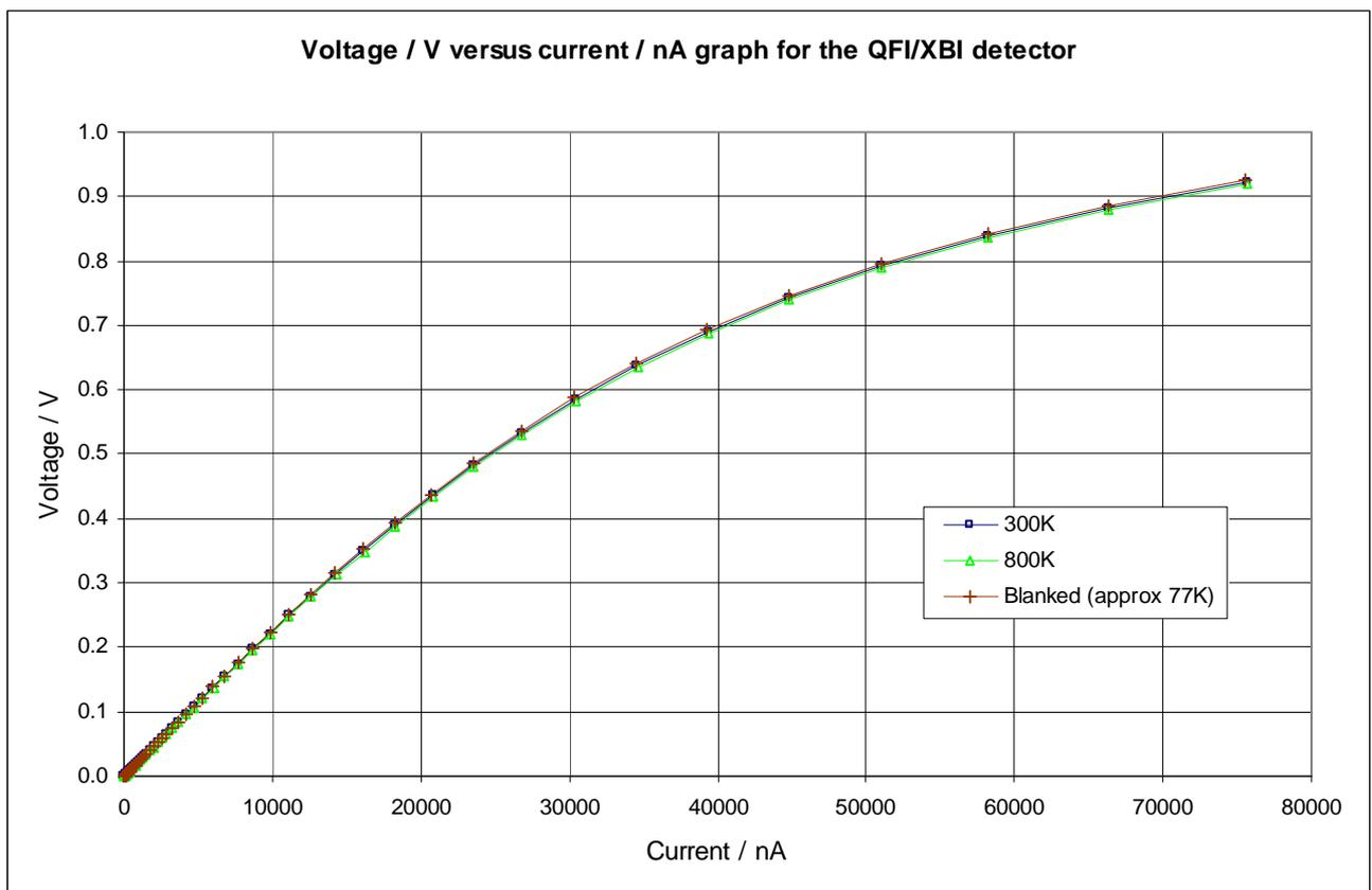
**Fig. 6.3.** The detector system VI characteristic measured with 77K, 300K and 800K dc loads
