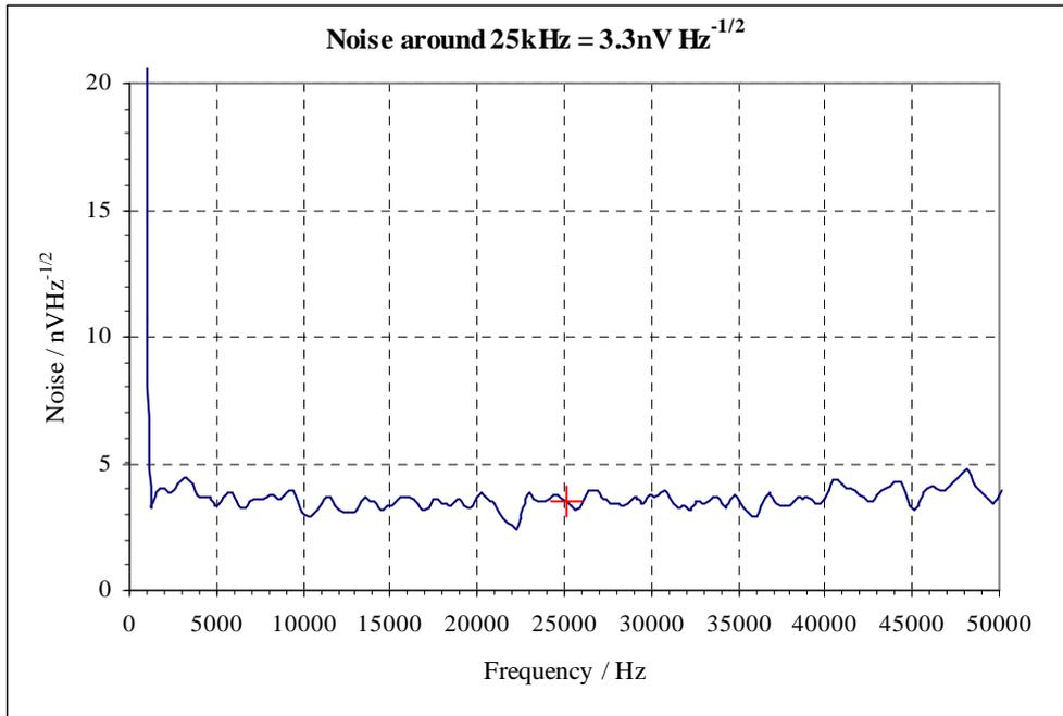
**Fig. 6.2b.** System output noise spectrum for the InSb detector 0 to 50kHz
