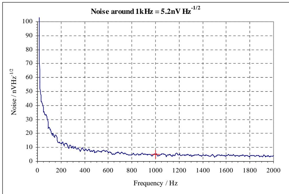
**Fig. 6.2a.** System output noise spectrum for the InSb detector 0 to 2000Hz
