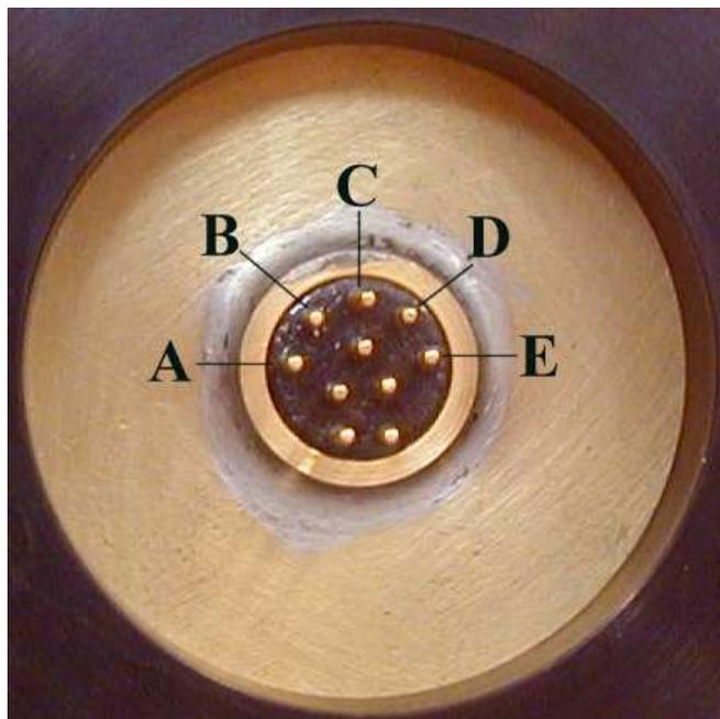
**Photo 4.4.** Electrical port pin assignments. InSb detector attached to pins D-E
