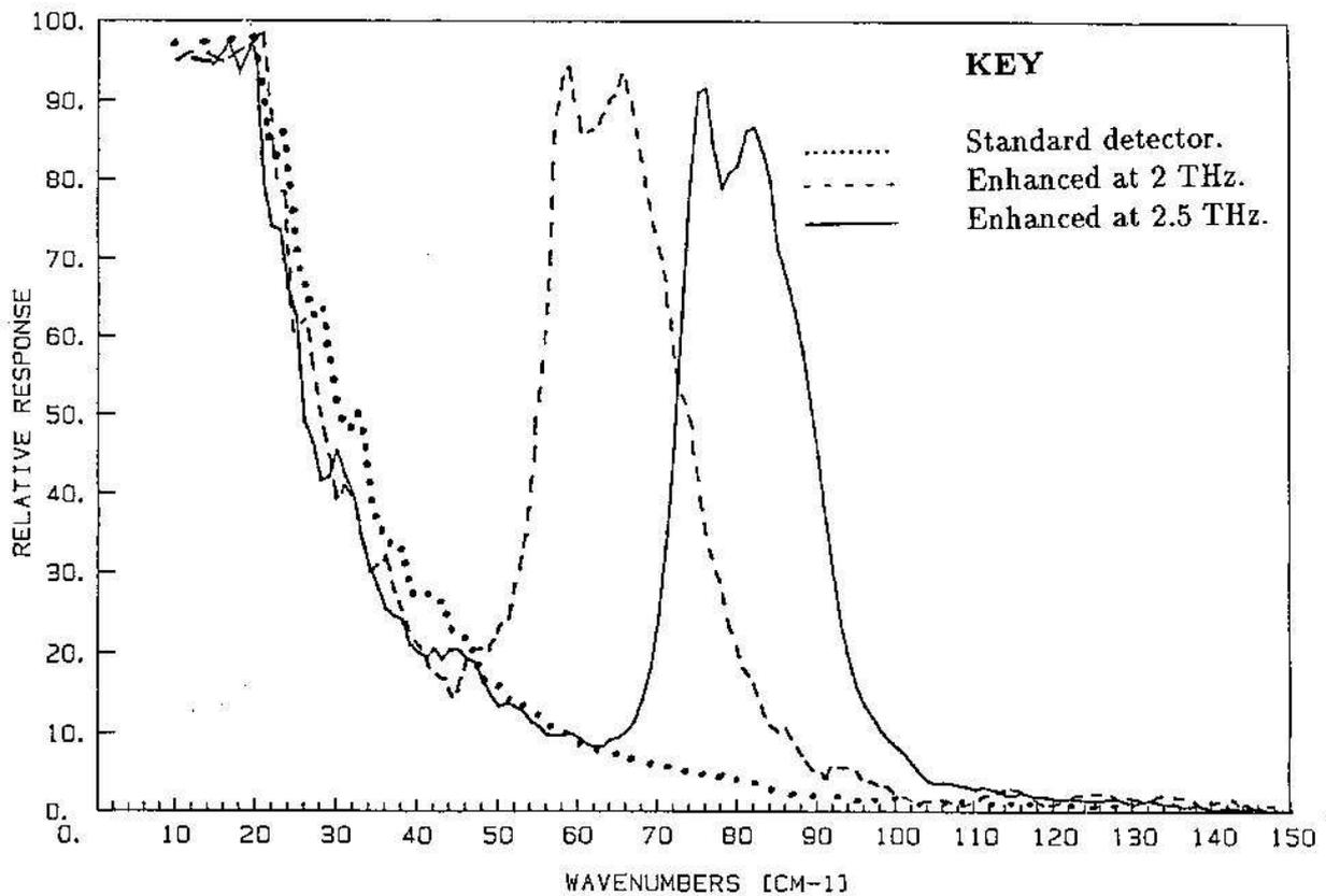
**Fig. A.1.** Spectral responsivity of a QFI/X detector with no magnetic field applied and two examples of type QFI/XB detectors enhanced at 2THz and 2.5THz
