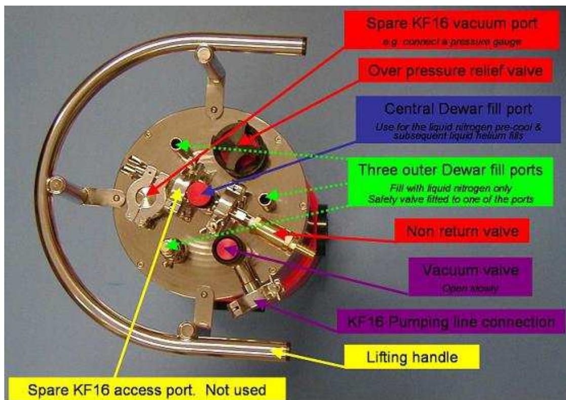
**Photo 2.1.** TK1813 cryostat top-plate fittings
