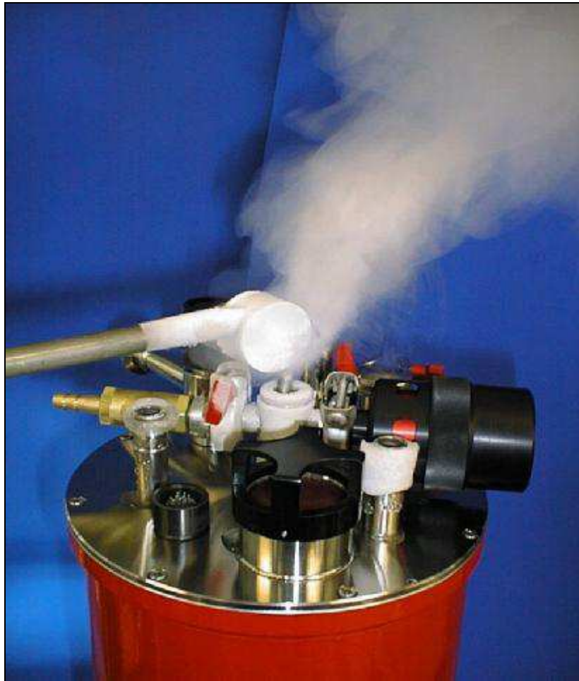
Photo 4.3. Helium plume when complete
