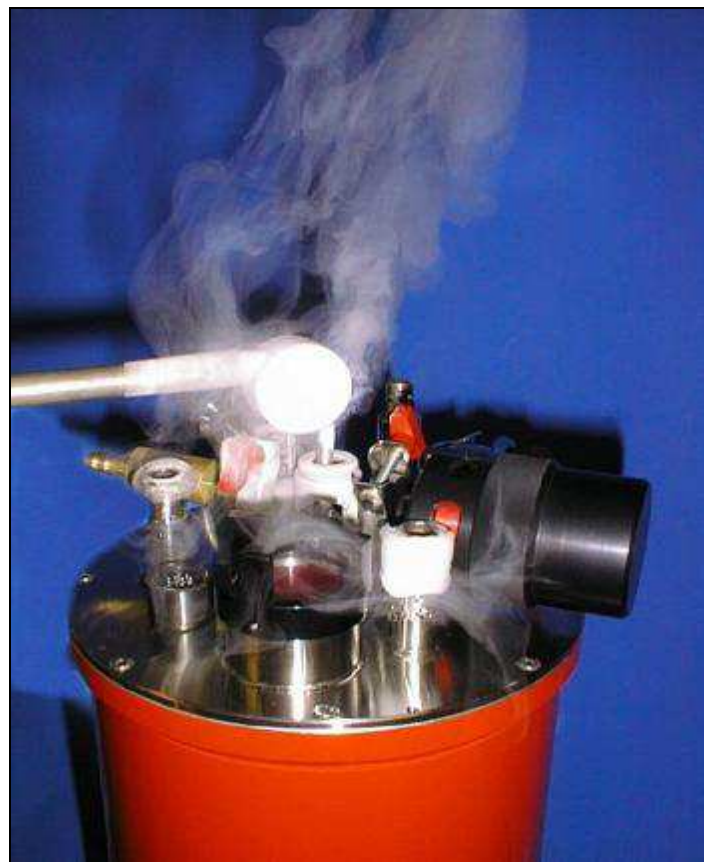
Photo 4.2. He gas exhaust during fill
