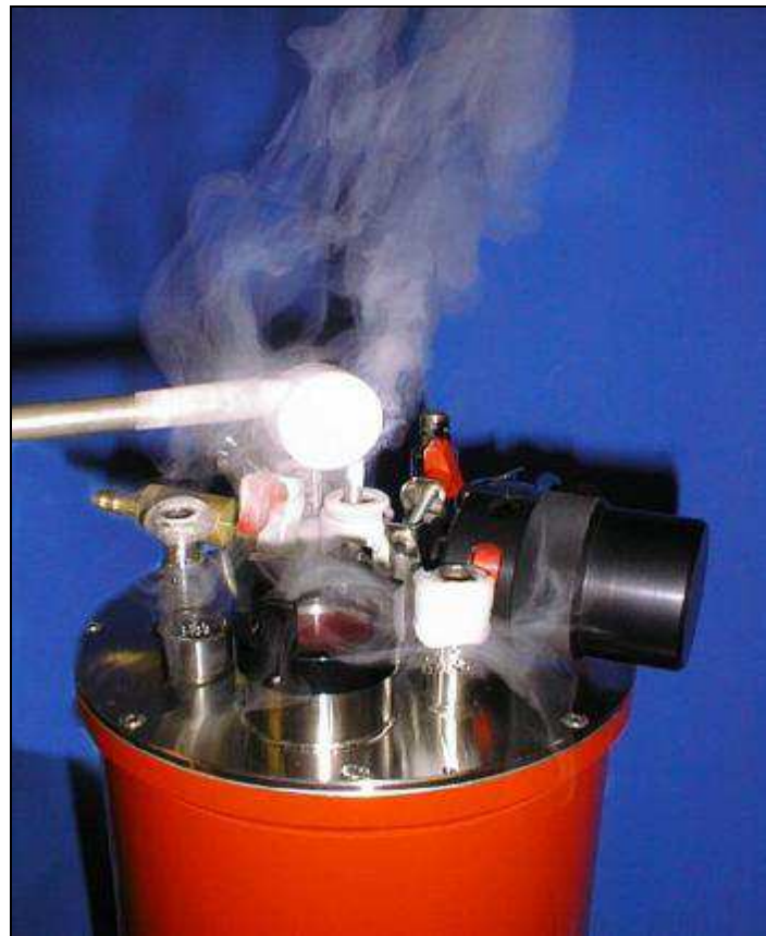
Photo 4.2. He gas exhaust during fill
