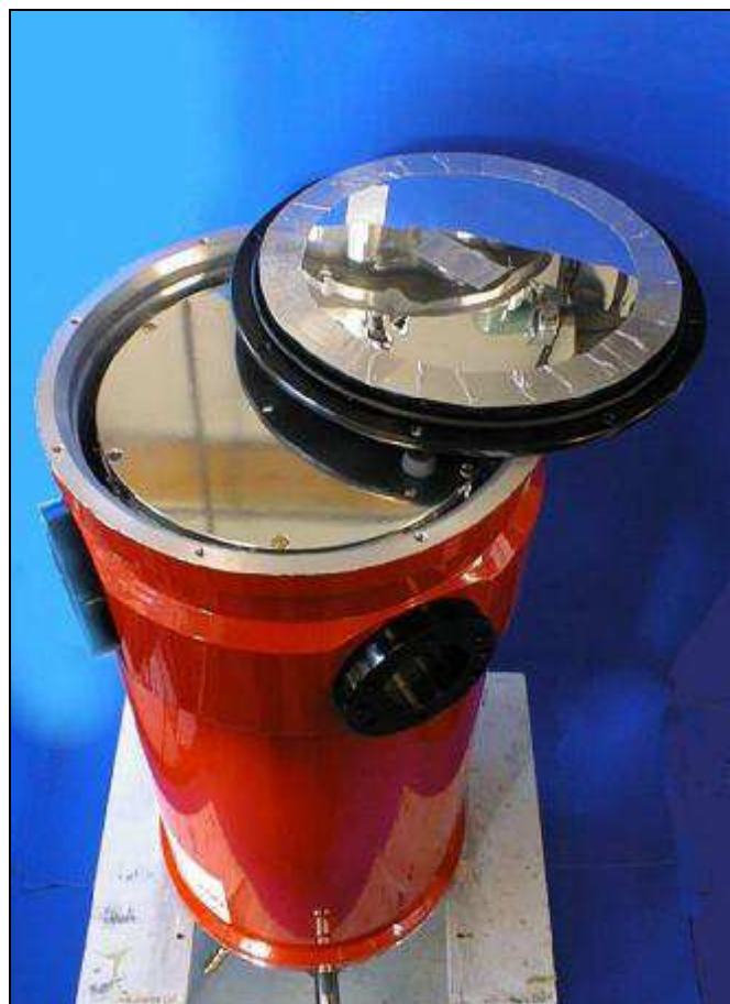
Photo 1.4. Liquid N 2 base plate in position
