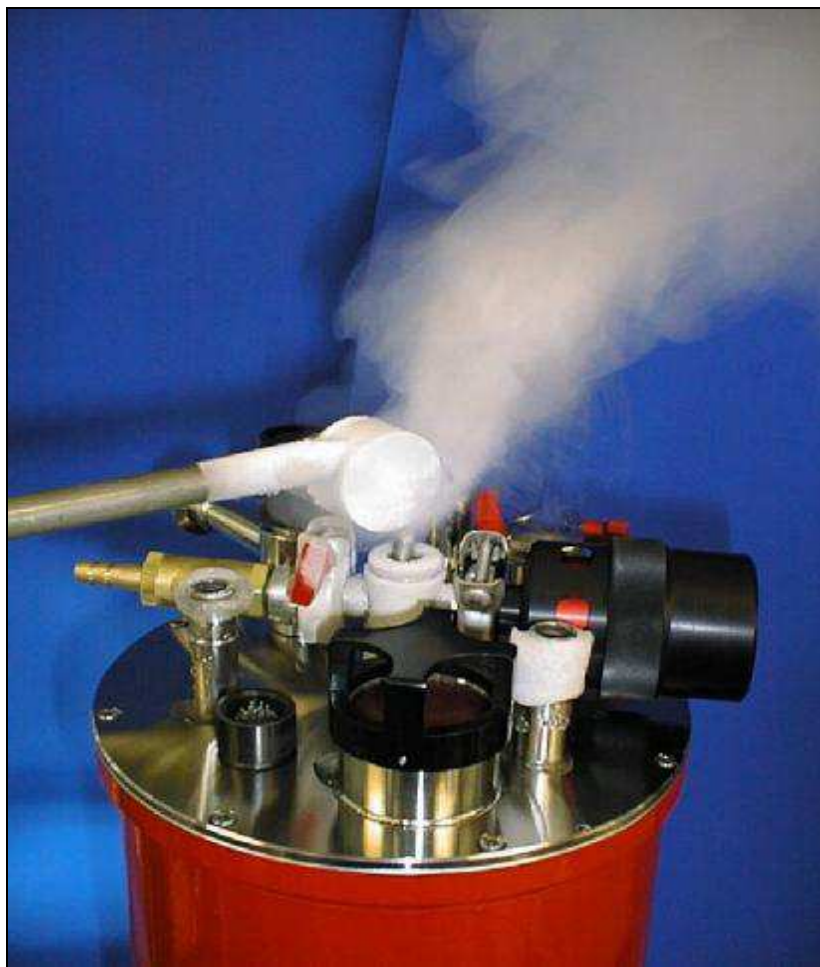
Photo 4.3. Helium plume when complete
