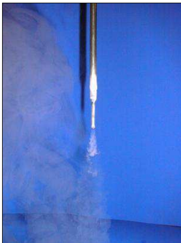
Photo 4.5. LHe emerging from a cold tube
