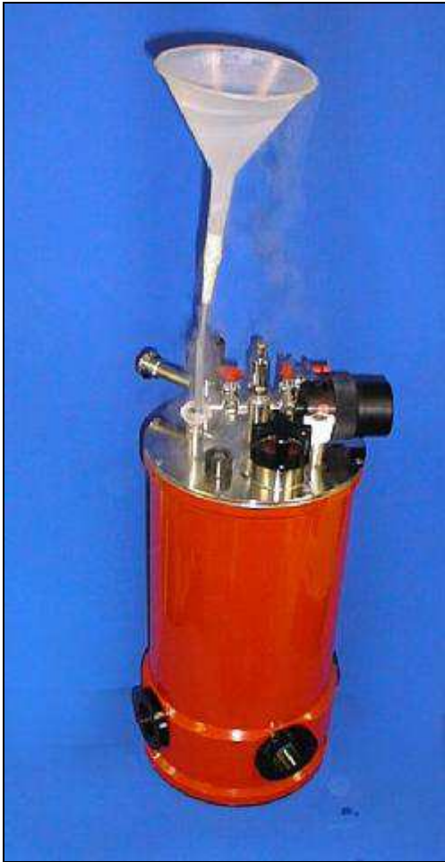
Photo 3.1. Using a funnel to fill the cryostat with LN 2
